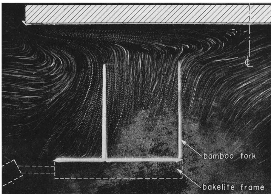
FIG. 21. Buoyant plume from a temperature probe ( \theta_w - \theta_\infty \doteq 100^\circ\text{C} ).
